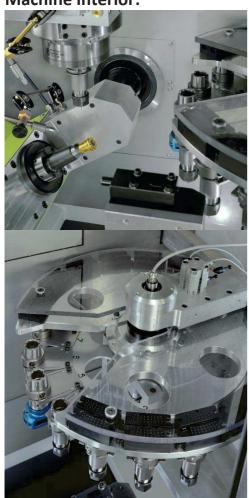
This 5-axes milling centre also offers a great deal of freedom and possibilities due to its design and its axle arrangement which are not possible with conventional milling centres. Especially rings, bangles as well as watch parts are diamond milled, engraved, facetted, etc. on any surface or in combination with our FourC, gemstones are set fully automatic.
