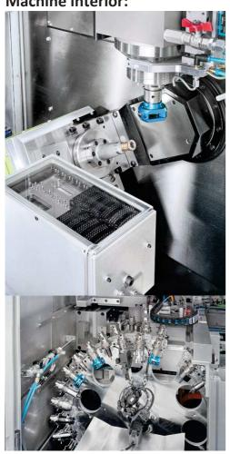
Due to its design and its axle arrangement, this 5-axes machining centre offers a great deal of freedom and possibilities which aren't possible with conventional milling centres. No matter wheter rings, bangles, jewellery or watch parts, any surfaces are diamond milled, engraved, guilloched, facetted etc. or in combination with our FourC, gemstones are set fully automatic.
